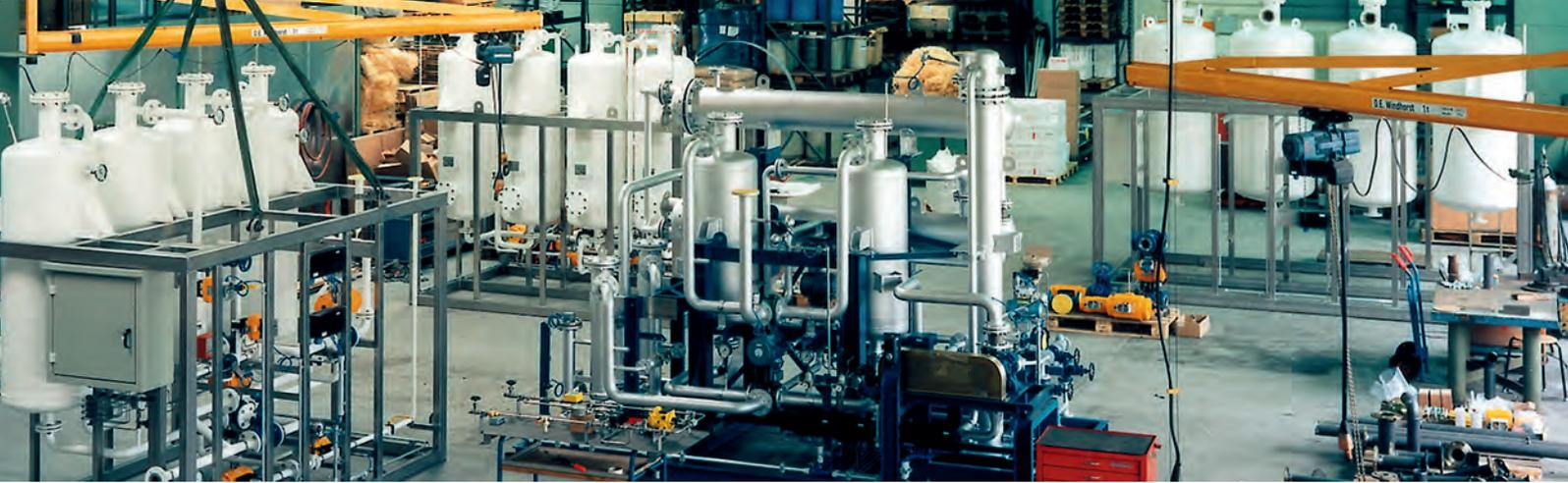
In most cases, the solvents flowing out of the separator can be re-used immediately. The solvents may still contain traces of water. In so far as this water prevents any reuse of the solvents, it can be dried with adsorbents such as Silica Gel or molecular sieves. If the solvent is water soluble, it is not possible to use simple separation techniques. Other methods involving processes such as distillation or rectification will have to be employed.
