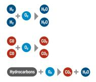
Upstream the reactor, sufficient oxygen resp. hydrogen, in special cases also carbon monoxide, is supplied to the gas to be purified. The reactor is filled with a palladium or platinum catalyst, where oxygen and hydrogen are oxydised to water resp. carbon monoxide to carbon dioxide.
